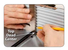
With your cutter-head and knife at "Top Dead Center" and using a square from the out feed table, mark your fence vertically in line with the knife as shown in photograph.
