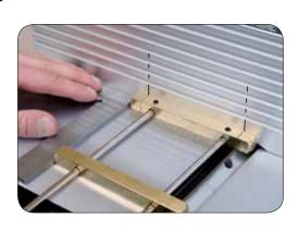
Place the Jointer Knife Setup Jig back onto your out feed table and align the two pre-scribed lines to the to lines on your fence. Next, place your square flat onto the table top surface and up against the jig. Square up the jig and secure the set screws with a hex key wrench. Remove the square - your jig is now ready to setup your jointer knives.
