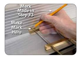
Place the Jointer Knife Setup Jig onto your out feed table top so the brass bar with the two scribed lines is firmly against the fence. Align the right scribed line on the brass setup jig with the mark made on your fence in step #3. Once aligned, make a mark on your fence corresponding with the left scribed line on the brass setup jig as shown in the photograph.
