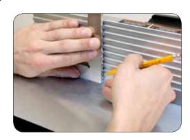
Remove the setup jig. Place your square up against the fence in line with mark made in step #4. Once aligned, mark or scribe a line on your fence as shown in the photo. You now should have two scribed lines on your fence that correspond with two scribed lines on the brass setup jig.
