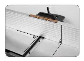
With the power dis-connected from the power source, adjust your jointer fence so that it is to the rear of the jointer table. The Fence should be at 90° to the out-feed table. Most new jointers automatically align when secured, however older jointers may be "free floating" fence types which must be properly aligned before proceeding.
