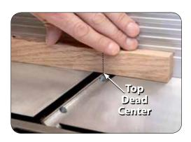
Find the Top Dead Center of your jointer knife by placing a straight edge on the out feed table over the jointer knife as shown in photo. Rotate the cutter-head until the knife just touches the straight edge. The spot where the knife contacts the straight edge is the Top Dead Center of your cutter-head. **Shop Note:**
