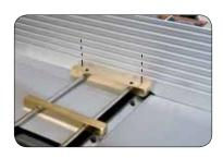
Insert the jointer knife into the cutter-head. Next, place the setup jig back onto the table and align the jig to the marks previously made as shown in step #6. Rotate the cutter-head until the magnets on the jig pull the knife up to the jig. Once the knife is against the magnets, be sure the knife tip is aligned with index mark made in step #3. Secure your knife and repeat this process for all remaining knives.
